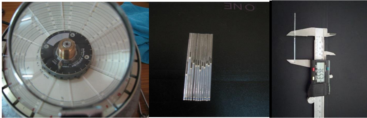
Figure 1. Measuring milk fat in elephant milk samples (as a percentage of total sample) using a simplified centrifugation technique and calipers, suitable for field sampling.
