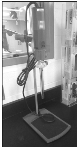
Figure 1. An example of a homogenizer, VWR model VDI 25 S41
