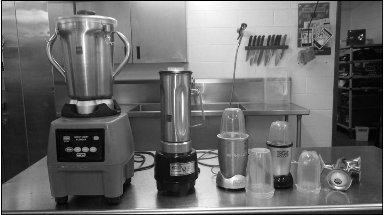
Figure 2. From left to right: Waring Heavy Duty CB15 4 L capacity, Waring HGB160 2 L capacity, NutriBullet® with a tall cup next to it, Magic Bullet® with a tall cup next to it, 10 lb manual meat grinder.
